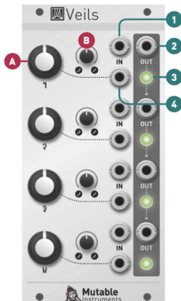
**A. Gain CV amount.** Amount of gain (amplitude) modulation from the CV input (4), or direct gain control when no cable is patched in the CV input. When this knob is turned fully clockwise, a CV of +5V yields a
