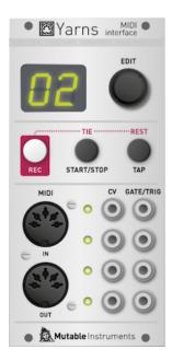
At the right of Yarns' display is an encoder which is used to increment/decrement values and scroll through options. The typical way of modifying Yarns' settings is to scroll through the list of settings, click
