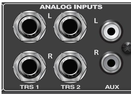
These inputs are for your audio sources (mixer, audio interface, CD player, etc.). Only balanced cables should be used when connecting the balanced TRS inputs of your Central Station to these devices. Because of the Central Station's passive circuitry, using unbalanced cables can reduce the output level and can introduce noise into your system.
