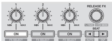
Beat FX turns on and off each time the button is pressed.
