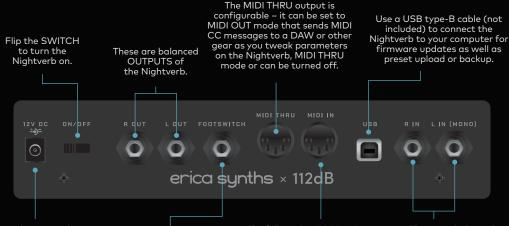
Connect the external POWER SUPPLY here! Use only the PSU that came with the unit, otherwise you risk damaging the Nightverb permanently.
