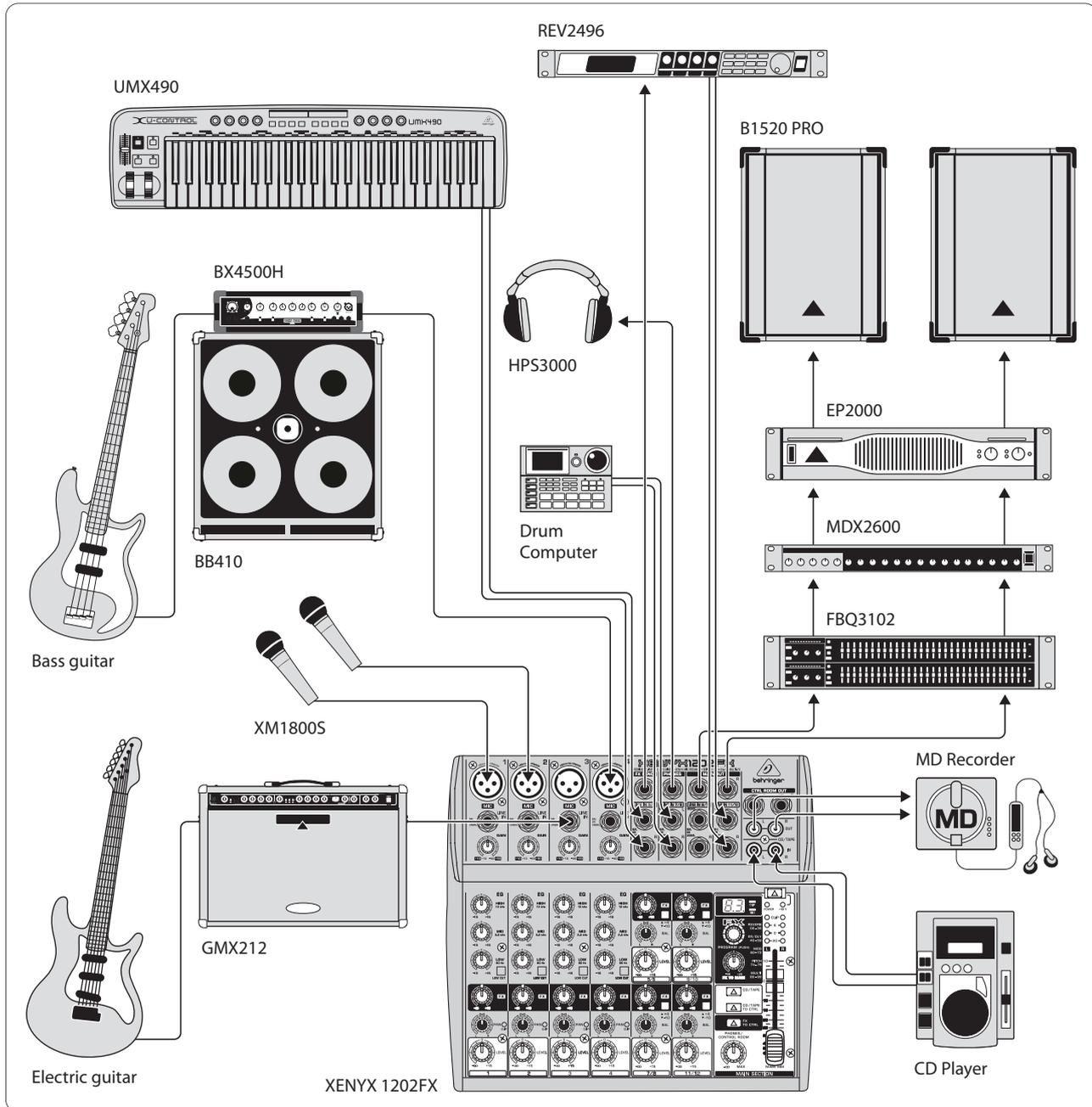
Fig. 3.2: Live application of the 1202FX
