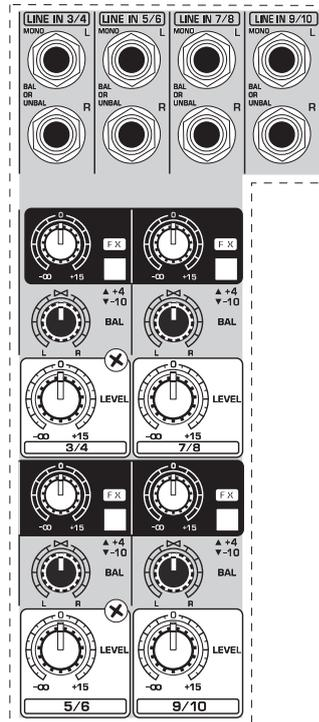
Fig. 2.2: Connectors and controls on the stereo channels
