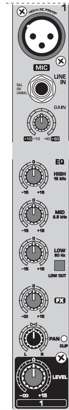
Fig. 2.1: Connectors and controls on the mono channels
