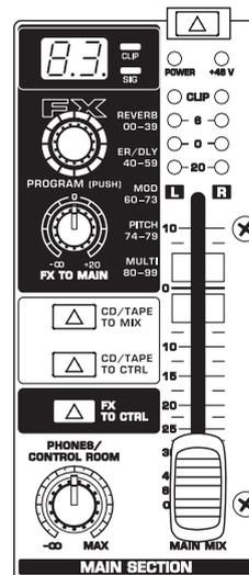
Fig. 2.4: Control elements of the main section
