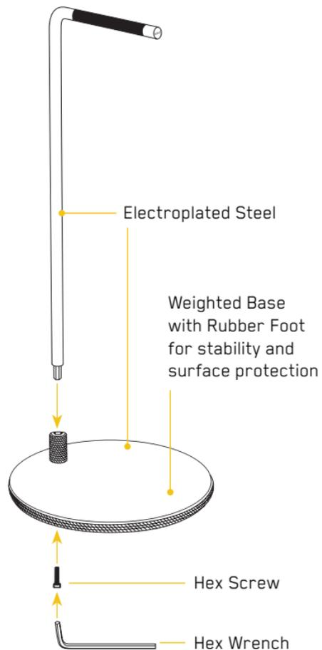
**ASSEMBLY:** Insert the end of the stand arm into the weighted base.
